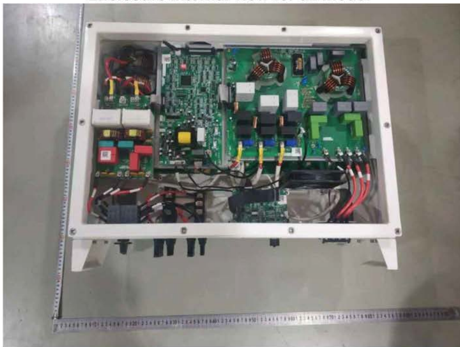
Enclosure internal view for all model
