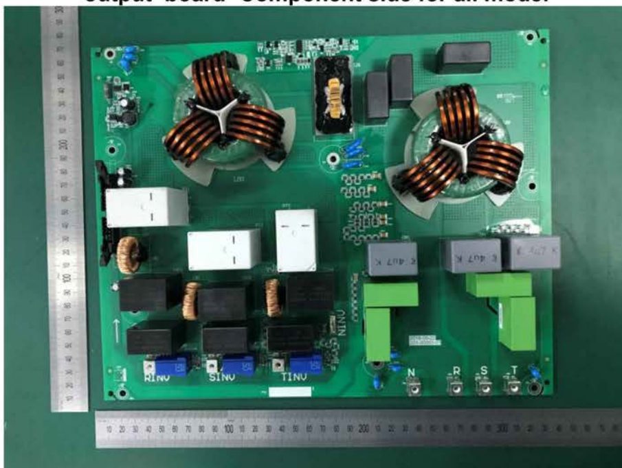
output board- Component side for all model
